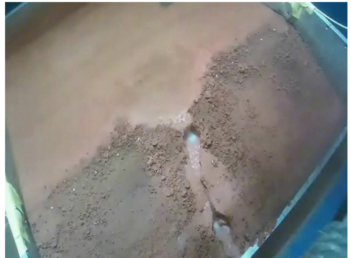
Figure 1. The headcut phenomena were occurred during dynamic load test on levee using centrifuge
